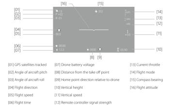
▲ If [04] and [09] both point in the same direction, the drone is flying towards to remote controller/home point.
