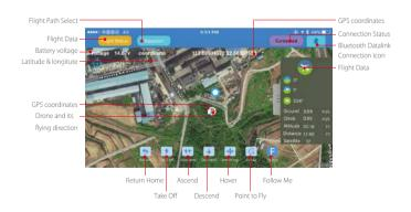
4. Once you have a minimum of 9 GPS satellites, you can unlock the drone and start flying with controller, or use the APP to unlock the motors and start flying.
